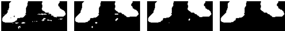
Figure 9: Segmentation result with different number of iterations j=0,2,4,6 (from left to right) during the MRF-computation.
