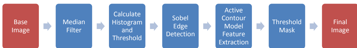
Figure 13 : Proposed Method for Processing an X-ray Image
