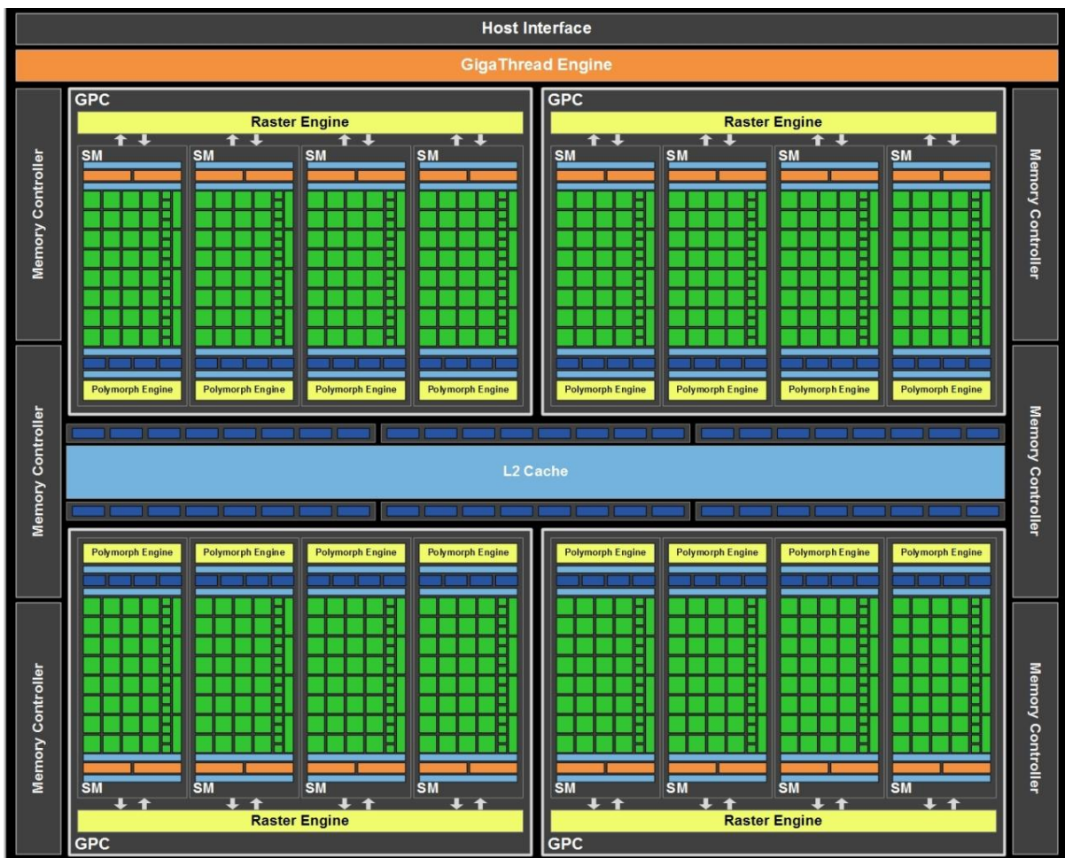
Figure 9 : Nvidia GeForce GTX 580 GPU Architecture
