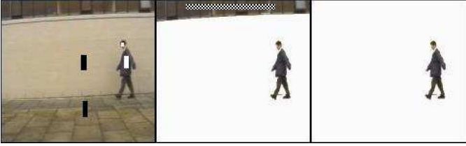
Fig. 6. Segmentation in Videos using user seeds. The first image shows one frame of the input video with user segmentation seeds (the back and white boxes). The image pixels contained in these boxes are used to learn histograms modelling foreground and background likelihoods. The second image shows the segmentation result obtained using these likelihoods with the method of [4]. The result contains a certain portion of the background wrongly marked as the foreground due to similarity in colour. This error in the segmentation can be removed by the user by specifying a hard constraint. This involves marking a set of pixel positions in the wrongly labelled region as background (shown as the checkered region in the second image). This constraint is used for all the frames of the video sequence. The third image is the final segmentation result.
