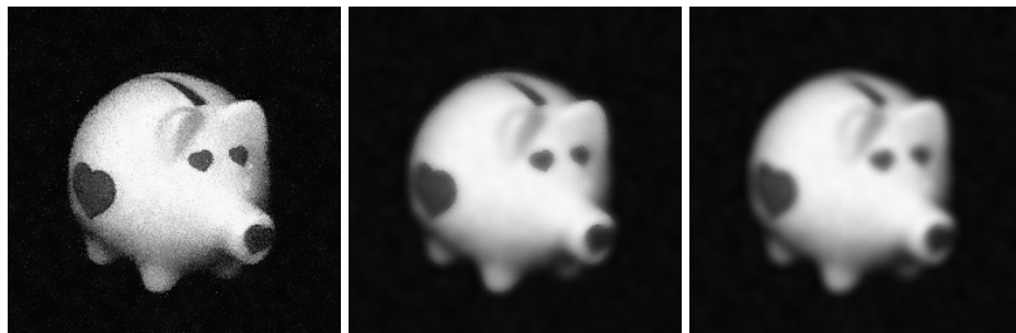
(g) \sigma_S = 5.0 et \sigma_I = 0.1 , PSNR=26.8 dB MSSIM=0.29 (h) \sigma_S = 5.0 et \sigma_I = 0.5 , PSNR=26.8 dB MSSIM=0.37 (i) \sigma_S = 5.0 et \sigma_I = 1.0 , PSNR=25.9 dB MSSIM=0.36
