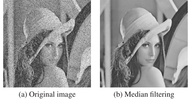
Figure 7. O(1) median filtering. (a) is the original image and (b) is our median filtering result which is the same as exact.
