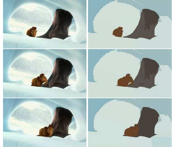
Figure 5: Video segmentation. Left column, input video ( 600 \times 480 \times 50 ), from top to down, 1th frame, 28th frame, 50th frame. Right column, segmentation results.
