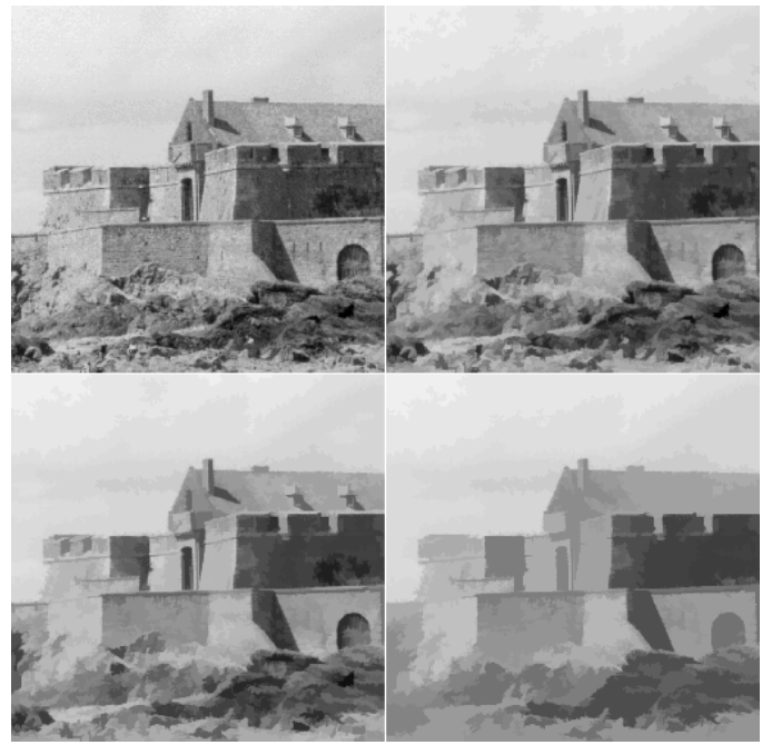
Fig. 12. Up-left: original image 256x256, Up-right: image at scale 10 (all shapes having area less than 10 pixels are removed), Down: image at scale 40, and 800 (sum of the CPU time for the 3 processed image: 0.38 s on a P200MMX).
