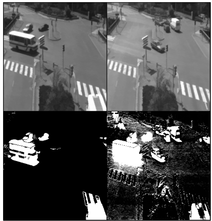
Fig. 16. Comparisons of images. Up: two original images. Down: The quantized image (left) reconstructed from the shapes of image 1 having no similar shape in image 2 and a quantized pixel by pixel difference of the images (right).
