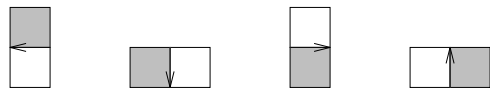
Fig. 10. The usual way the local configuration of the border of a region is coded. In each figure, the pixel inside the region is the dark one. The border is indicated by inter-pixel directions, always leaving the region to the right.
