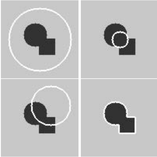
Figure 12.1. A simple case, showing that the fitting term E_1(\Gamma) is minimized when the curve is on the boundary of the object.
