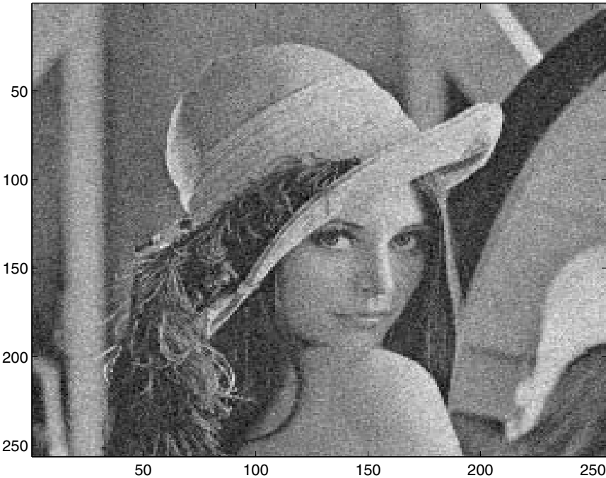
Figure 11.5. Noisy image, signal-to-noise ratio approximately equal to 3.
