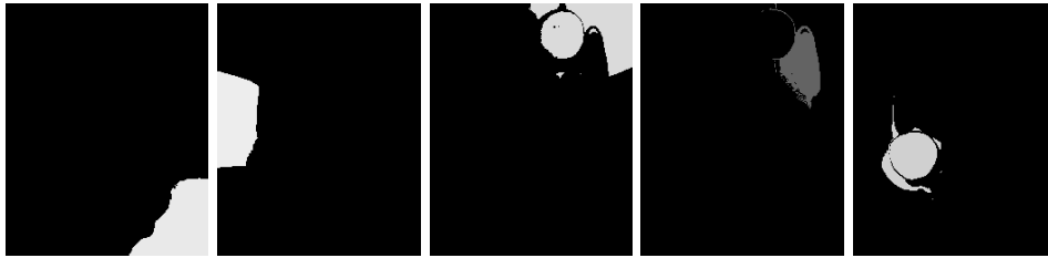
Figure 16.16. Five of the segments obtained by segmenting the image of vegetables with a k -means segmenter that uses position as part of the feature vector describing a pixel, now using 20 segments rather than 11. Note that the large background regions that should be coherent has been broken up because points got too far from the center. The individual peppers are now better separated, but the red cabbage is still broken up because there is no texture measure.
