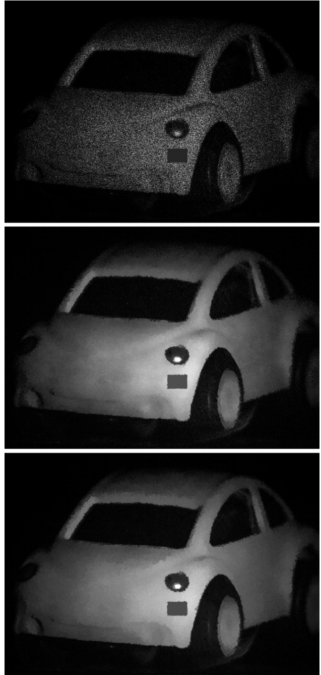
Fig. 11. Top, reference image of a toy car reconstructed from an experimental digital hologram of 1123 \times 1585 pixels with first-order speckle (or one look), drawn with modification of gray levels for visualization. Middle, result with 3-pixel base triangle, \mu = 5.0 and \beta = 0.3 (260 s, 889,978 nodes, PIII-1.1 GHz). Bottom, result with 5-pixel base triangle, \mu = 5.0 and \beta = 0.3 (61 s, 222,437 nodes, PIII-1.1 GHz).
