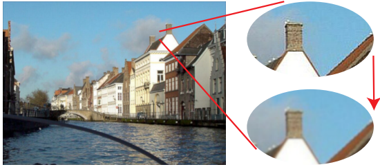
Figure 5: The Gaussian filter give much smoother results compared to the box filter. We have applied a 7 \times 7 filter to the above image two times. The result preserves important details of the original image while the noise is effectively eliminated.
