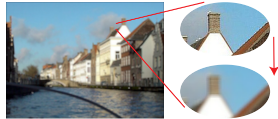
Figure 3: A 9 \times 9 box-filter is applied to the image. As the filter is not smooth, the blocks are still visible after a relatively wide kernel.
