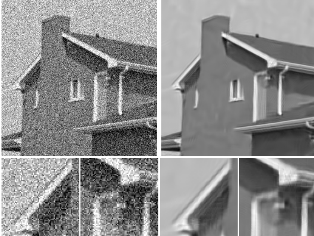
Figure 4. On the left are a noisy ( \sigma = 35 ) House and two enlarged fragments from it; on the right are the denoised image (PSNR 31.21 dB) and the corresponding fragments.
