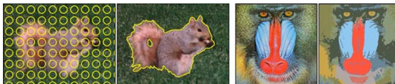
Figure 3. Binary segmentation of a color image using multivariate Gaussian distributions as region descriptor (initialization and final segmentation) and multiphase color segmentation obtained with the algorithm developed in Brox and Weickert (2004)
