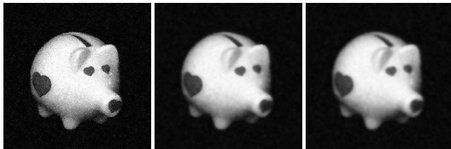
(d) \sigma_S = 2.0 et \sigma_I = 0.1 , PSNR=26.7 dB MSSIM=0.29 (e) \sigma_S = 2.0 et \sigma_I = 0.5 , PSNR=27.9 dB MSSIM=0.39 (f) \sigma_S = 2.0 et \sigma_I = 1.0 , PSNR=27.5 dB MSSIM=0.38
