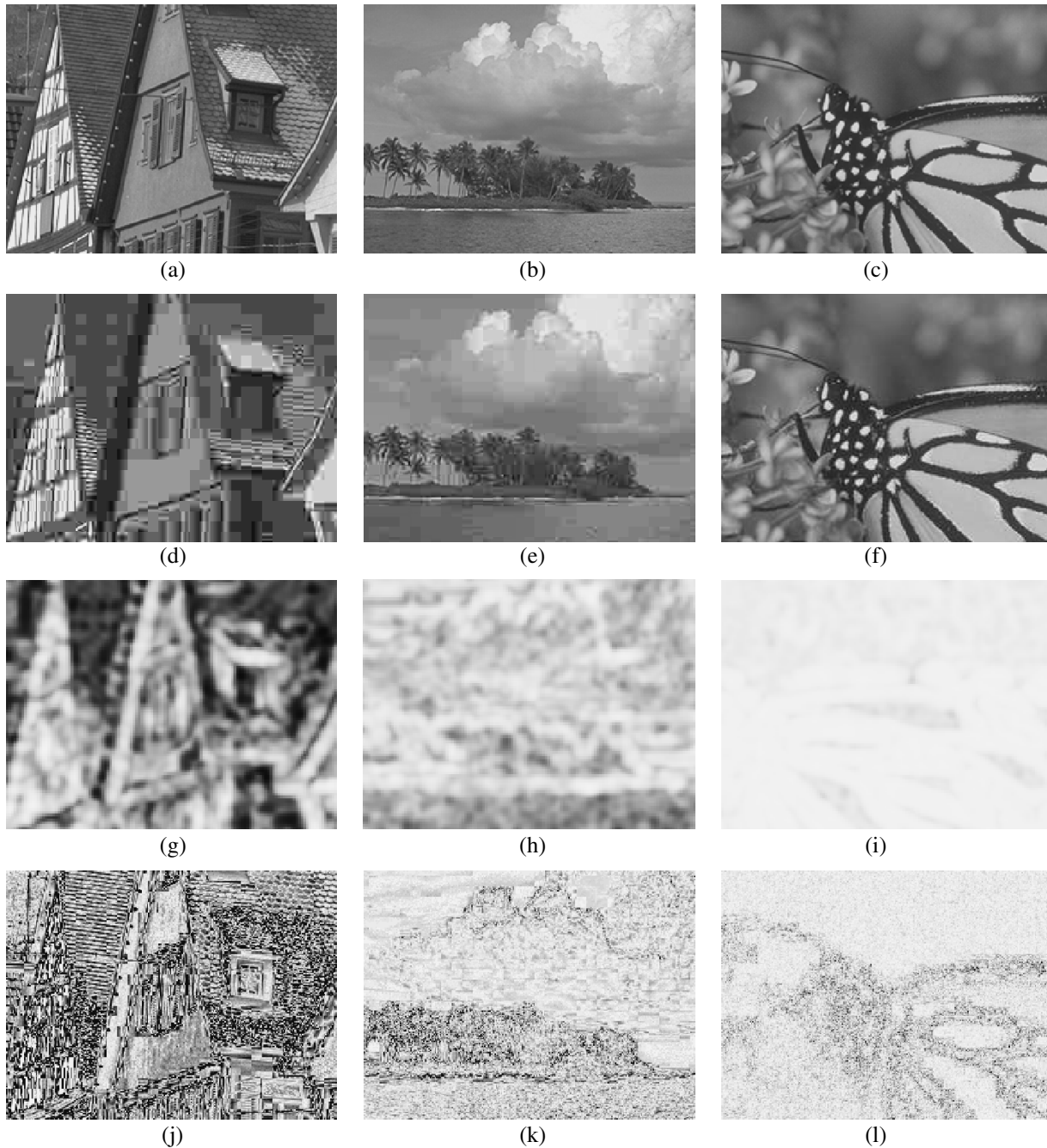
Fig. 6. Sample JPEG images compressed to different quality levels (original size: 768 \times 512 ; cropped to 256 \times 192 for visibility). The original (a) “Buildings,” (b) “Ocean,” and (c) “Monarch” images. (d) Compressed to 0.2673 bits/pixel, PSNR = 21.98 dB, MSSIM = 0.7118. (e) Compressed to 0.2980 bits/pixel, PSNR = 30.87 dB, MSSIM = 0.8886. (f) Compressed to 0.7755 bits/pixel, PSNR = 36.78 dB, MSSIM = 0.9898. (g), (h) and (i) show SSIM maps of the compressed images, where brightness indicates the magnitude of the local SSIM index (squared for visibility). (j), (k) and (l) show absolute error maps of the compressed images (contrast-inverted for easier comparison to the SSIM maps).
