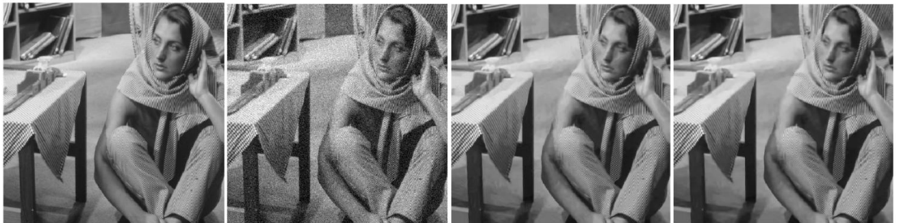
Figure 4. Denoising Results. (1) Original noiseless image. (2) Image with Gaussian noise, \sigma=25 , (3) Denoised image using the BM3D, (4) Denoised image using the ensemble learning
